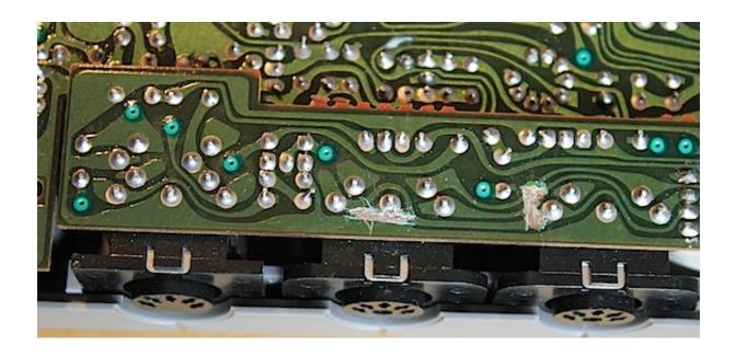
Solder 2 wires, if you want, you can scrape some green mask of the PCB . Don't use leadfree solder here!
